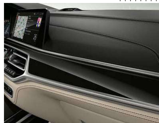
A brilliant appeal: The deep shine of the BMW Individual interior trim finishes in piano finish Black is the result of an elaborate process in which several layers of wood veneer are applied and then painted and polished in numerous layers with piano finish. The result: a unique surface that shines with noble brilliance.
